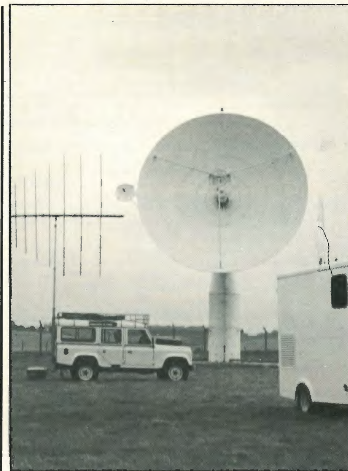
Monitoring equipment at the Department of Trade's station near Baldock in Hertfordshire, which can cover the spectrum from 10kHz to over 12GHz.
